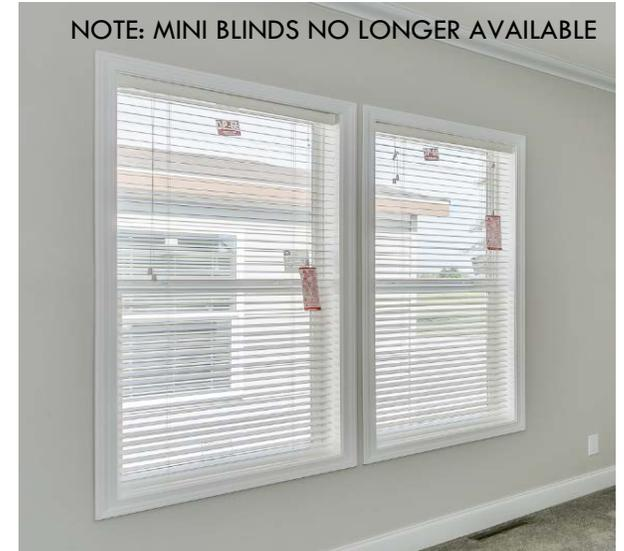
2 1/4" 4Y WINDOW AND DOOR CASING WITH 5/8" WRAPPED STYLE JAMBS
